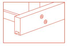
Tighten fasteners to secure the fixed shelf to the wood supports
