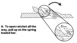
B. Keeping the spring loaded bar compressed, open ratchet all the way.
