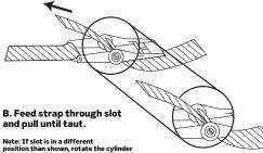
Note: If slot is in a different position than shown, rotate the cylinder by hand until it is at a 45° angle, or so you can easily feed the strap through the slot as shown.
